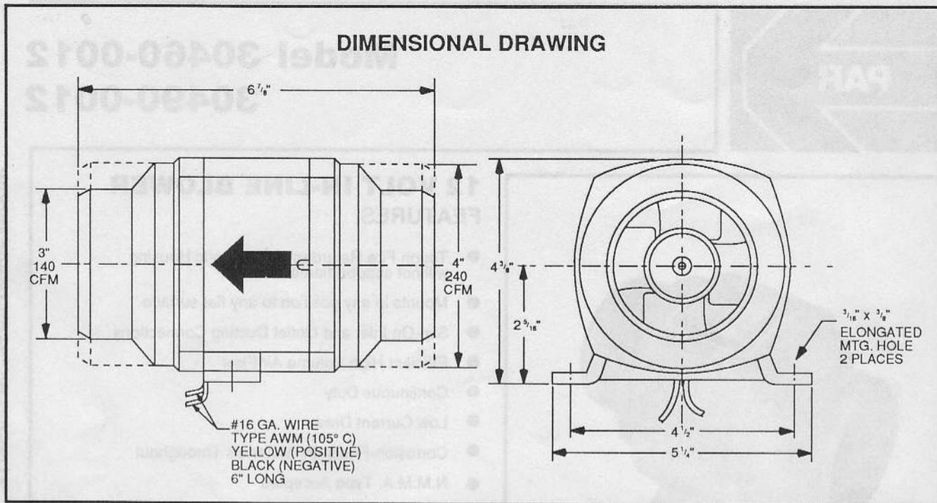
**OPERATION:** The blower may be used for continuous operation. However, maximum motor brush life is generally about 1000 hours.
