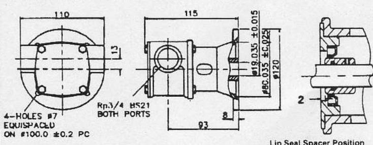
**Suitable For** (a) 80-B3/B14 Motor Frame To IEC Std
