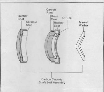
Remove marcel washer, carbon ring assembly, and seal seat with a hooked wire. Use care not to scratch shaft or seal seat bore. Inspect shaft and seal seat bore to be sure sealing surfaces are free of wear tracks, nicks or scratches. Clean shaft surface behind splines to insure proper O-ring seal on shaft.
