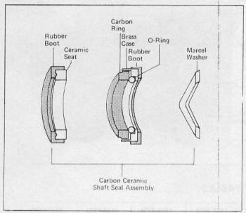
Remove marcel washer, carbon ring assembly, and seal seat with a hooked wire. Use care not to scratch shaft or seal seat bore. Inspect shaft and seal seat bore to be sure sealing surfaces are free of wear tracks, nicks or scratches. Clean shaft surface behind splines to insure proper O-ring seal on shaft.
