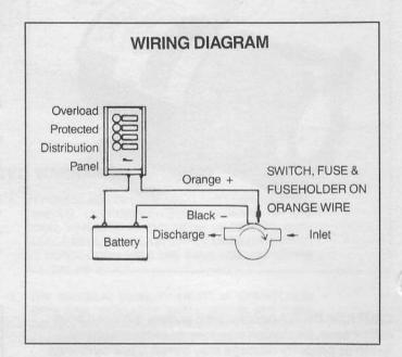
NOTICE: No warranty consideration will be given to pumps that are returned without the properly sized fuse and fuse holder supplied with the pump.
