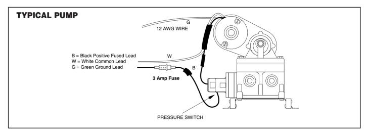
These pumps with 115 Vac rectified motors meet USCG Regulation 183.410 and ISO 8846 MARINE for Ignition Protection.
