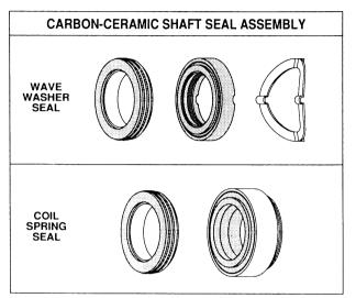
Older models of this pump were fitted with a shaft seal that was compressed by a wave washer type compression spring. When replacing this older seal assembly with a new style seal that is compressed by an integral coil type spring, remove and discard the wave washer.
