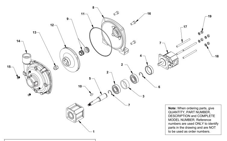
Note 1: Mechanical Seal Ref. 9 is not available outside of the kit form. For replacement seal, order Kit #3430-0332 or Kit #3430-0589 for Model 9302CT-GM1 and Kit #3430-0589 for
