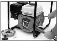
4. Between the impeller and casing cover is the mechanical seal. On the backside of the impeller is the seal's ceramic seat. If either part of the seal is damaged, with cracked or scuffed surfaces, the seal will fail to perform satisfactory and will leak. To remove the seal seat from the impeller, use a small blade screwdriver and wedge
