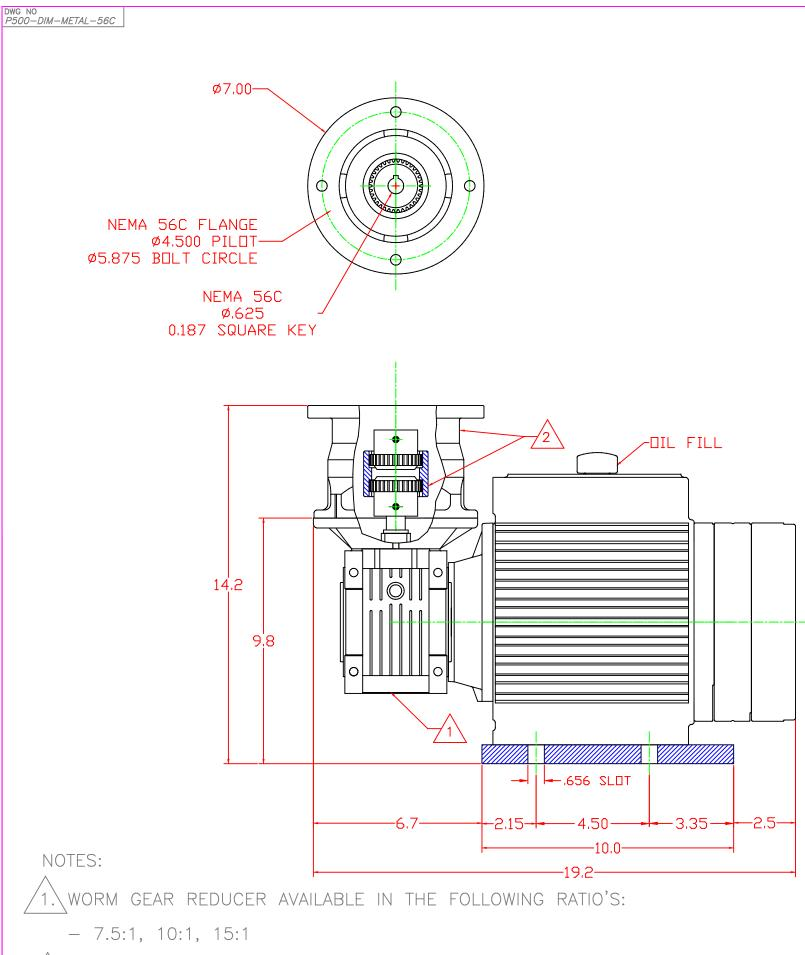
2. MOTOR ADAPTER AND COUPLING REQUIRED FOR USE OF 56C MOTOR.
