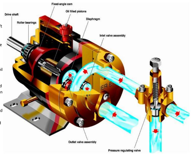
To provide long trouble free diaphragm life, the Hydra-Cell™ hydraulically balances the diaphragm over the pump's complete pressure range. The diaphragm actually faces only a 2 PSI pressure differential no matter at what pressure the fluid is being delivered.
