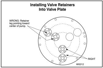
e. Inlet (3 center valves). Insert the three remaining spacers (15) into the inner ring of valve bores in the valve plate. The flat, flanged end must be facing down toward the shoulder of the valve plate.
