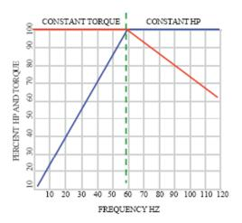
Variable Frequency Drive (VFD): An electronic controller that adjusts the speed of an electric motor by modulating the power being delivered. A constant volts/Hz relationship is maintained from 0-60 Hz, while voltage is typically held constant above 60 Hz. See chart above for implications on motor torque and horsepower output:
