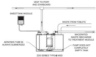
INCLUDES HOLDING TANK WITH LEVEL MONITOR
