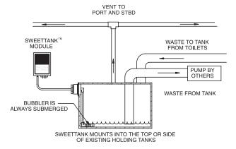
Install a complete ZDS Series Type-III MSD. ZDS includes the holding tank, level monitor, macerator/discharge pump and SWEETTANK<sup>®</sup> (see Page 48).
