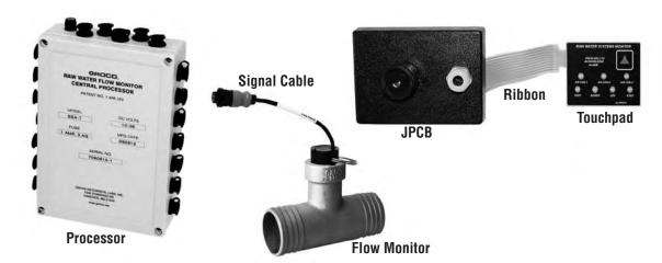
**The Concept:** GROCO® SSA-7 continuously monitors raw water flow to as many as seven devices (engines, generators, air conditioners, refrigeration, R/O systems, pumps, etc). Through calibration the patented process considers unique individual plumbing and flow parameters, and learns "normal" flow for each connected device. Audible and visual alerts are provided within 7 seconds of a dangerous reduction of raw water flow to any of the devices.
