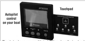
The photo shows one possible installation where the touchpad ribbon runs through an existing hole behind the autopilot control.
