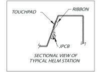
If you cannot route the large connector to the Processor you must cut the connections inside JPCB. Cut all wires about 1/2" from the terminal block leaving the wires connected and the colors visible. This will aid with re-connection of the wires. Connect the large connector to the Processor, and run the cable to JPCB. Figure-2 Schematic shows proper wire connections.
