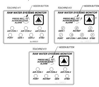
The touchpad has two buttons – an "acknowledge" (bell) button and a hidden button located next to the bell button. Lightly pass your finger over the hidden button location to detect a slight bump. Both buttons will be used during calibration.
