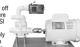
**WINTERIZATION:** Freezing will damage your pump and the connected plumbing. To winterize first allow PSR to pump the supply tank(s) dry. Shut off power when the faucets begin to pass air. Disconnect inlet and outlet hoses to drain the connecting plumbing and remove WSB-1000 bowl. Pour an ounce or two of potable alcohol (your favorite scotch will do fine) into the pump. Reconnect the hoses to prevent evaporation. DO NOT use automotive antifreeze to winterize as it may be poisonous.
