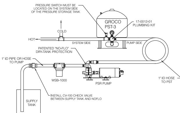
**INSTALLATION:** The motor and circuitry are not waterproof. Install PSR in a dry, well ventilated location not more than 10-feet above the water supply. If PSR will have a flooded inlet the pump may be oriented in any position; if PSR must self-prime orientation must be upright.
