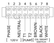
\* For 240V, remove jumper and supply power to terminals 1 and 2, with neutral on 3.
