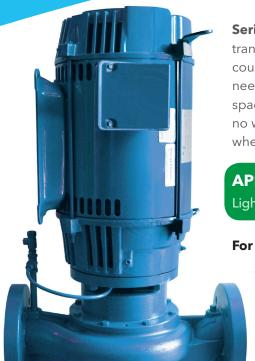
**Series A-C e-1500** is designed for light industrial and general water transportation. Made of rugged cast iron, this heavy-duty, in-line, close-coupled pump can be mounted horizontally or vertically, eliminating the need for special pads or foundations, making this option ideal where space is limited. Offered in a variety of sizes to meet all of your needs, it's no wonder why this pump's timeless design delivers quality performance wherever and whenever it's needed.
