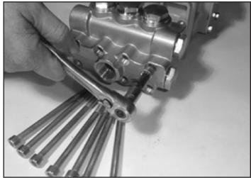
4. Remove hexagon socket screws (34) and remove valve casing (26) by pulling them frontwise over the plungers (16).
