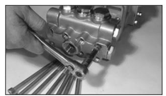
7. Remove hexagon socket screws (34) and remove valve casing (26) by pulling them frontwise over the plungers (16).
