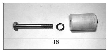
9. Check plunger surfaces (16). Damaged surfaces lead to accelerated seal wear. Deposits of all kinds must be removed from the plungers.
