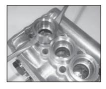
6) Remove seal adaptors (20) and weep return rings (25) from the valve casing.
