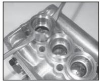
Remove seal adaptors (20) and weep return rings (25) from the valve casing.
