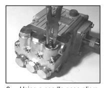
Using a needle nose pliers, remove the inlet and discharge valve assemblies (27-30), for P230-3100 only, remove spacer (30A), and o-ring (31). Inspect all parts for wear and replace as necessary.
