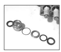
7. Remove the weep return ring (25), pressure ring (24), and v-sleeve (23) from the valve casing (26). Remove the rear v-sleeve (23A) from the seal case (20). Inspect all parts, including o-ring (21) for wear and replace as necessary.
