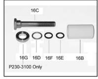
8.Check surfaces of plunger pipe (16B). A damaged surface will cause accelerated wear on the seals. Deposits of any kind must be carefully removed from the plunger surface. A damaged plunger must be replaced! When replacing the crush washer (item 16D), make sure the rolled side of the crush washer is placed on the ceramic. Prior to installation, carefully crush the seal ring on a hand press.
