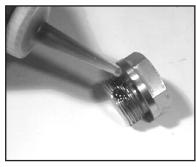
4. Apply one drop of Loctite 243 to the valve plugs (32) and tighten to 33 ft.-lbs.
