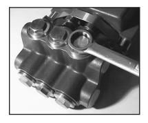
With a 27mm wrench, remove the three discharge plugs (#48) and three inlet plugs (#42A) from the manifold (#43).
