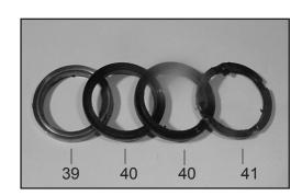
35. Reinstall the pressure ring (#39), v-sleeves (#40) and support ring (#41) into each plunger bore. Reinstall the tension spring (#42).
