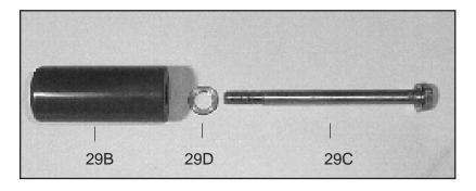
32. Inspect the ceramic plungers (#29B) and replace them if necessary. Clean the ends of the ceramic and remount onto the crosshead/plunger assembly. Make certain that the end of the plunger which is not counter-bored is facing the discharge side of the pump. Install the seal washer (#29D) on the bolt assembly.
