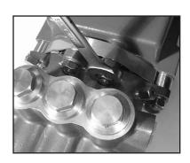
5. Remove the six manifold stud nuts (#50) with a 19mm wrench. Remove the spring washers (#50A). Tap the back of the manifold with a rubber mallet to dislodge and slide it off the studs (#49).
