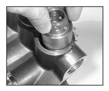
38. Reassemble the inlet valve assembly in the reverse order of step #7. Make certain all the components are press fit together and that the spring retainer (#54) is slightly counter sunk in the valve housing (#52). Grease the o-ring (#53) and install it on to the valve housing. Reinstall the entire inlet valve assembly into the manifold (#43). install the tension plugs (#42A) and tighten.
