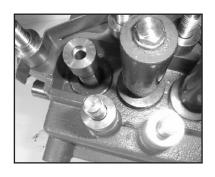
11a. Inspect the crankcase oil seals (#31) for evidence of leaking. If there is oil on the crankcase (#1) at the sight of the oil seals, they must be replaced. The oil seals are replaced after removing the crosshead/ plunger assembly (#25) as described below. Contact Giant Industries for service school information. Phone: (419) 531-4600
