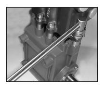
39. Lubricate the plungers (29B) again and slide the manifold (#43) gently and evenly over the plungers. Press the manifold firmly into place against the crankcase (#1). Install the spring washer (#50A) and tighten the manifold stud nuts (#50) to 696 inch-pounds (79 Nm).
