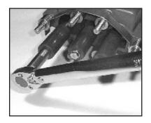
33a. Torque the ceramic plunger bolt assembly to 300 inch-pounds (34 Nm). If originally removed, reinstall the stud bolts (#49).
