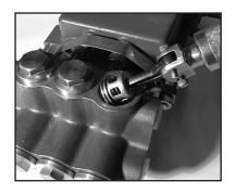
Using a valve puller (available from Snap-On-Tools), remove the valve assembly (#44 - #47).
