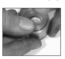
34. Install the rear support ring (#41), rear v-sleeve (#40), rear pressure ring (#39). Install the snap ring (#36).
