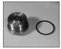
Inspect the plug o-rings (#48A and #42B) and replace as necessary.
