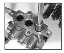
6. To remove the inlet valve assembly, insert a 13mm socket with extension through the rear of the inlet manifold (#43) port and tap it firmly with a hammer. This will force the tension spring (#46), valve housing (#52) and the remainder of the inlet valve assembly out through the front of the inlet port.
