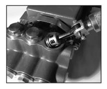
3. Using a valve puller (available from Snap-On-Tools), remove the valve assembly (#44 - #47).
