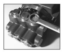
With a 27mm wrench, remove the three discharge plugs (#48) and three inlet plugs (#42A) from the manifold (#43).
