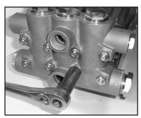
Loosen the 8 nuts (49A) with a 19mm wrench. Tap the back of the manifold (43) with a rubber mallet to dislodge and slide off the studs (49).
