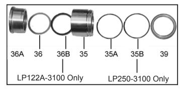
Lubricate seal (36). Place seal (36) and drip shield (36B for LP122A-3100 only), and pressure ring (36A) into the seal sleeve (35). Assemble the O-ring (35A) onto seal sleeve and lubricate. LP250-3100 has an additional O-ring (35B).
