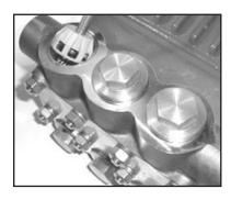
14. Next, place valve assemblies (46A) into manifold after first lubricating the O-ring (44A). Seat firmly into manifold.
