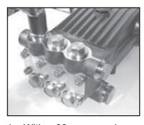
With a 30mm wrench, remove the six (6) plugs (48) from the valve casing (43). Inspect the o-rings (48A) and replace if necessary. Remove the complete valve assembly (46A) by threading a 12mm bolt into the spring retainer and pulling straight out.
