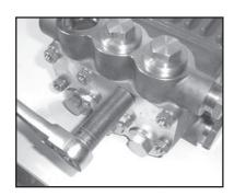
3. Remove the eight (8) hex nuts (49A) with a 19mm wrench. Tap the back of the manifold (43) with a rubber mallet to dislodge and slide off the studs.
