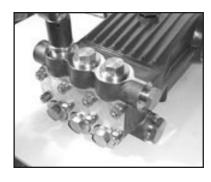
15. Replace plug with O-ring (48, & 48A) and tighten to 160 ft.-lbs. (217 Nm).
