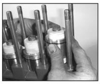
Press seal sleeve assembly into the manifold and seat firmly. Put the support ring (41) on plunger with v-side facing the manifold.
