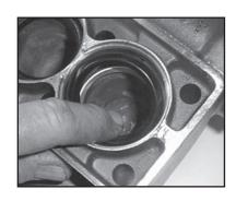
Place support ring (41) and v-sleeves (40) into valve casing. For LP250-3100, the support disc (37) is placed in the manifold before the support ring.
