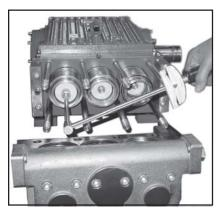
9) Coat the seal sleeve(39) lightly with anti-corrosive grease (e.g. molycote no.Cu-7439) in its fitted area towards the crankcase. Insert the seal sleeves in to their crankcase fittings. Coat the threads of the tension screw (36C) lightly with thread glue and insert it together with a new copper ring (36D) through the ceramic pipe. Turn the pump by hand until the plunger (25) rests against the plunger pipe. Tighten the tension screw at 30 Ft-lbs. (40 NM)
