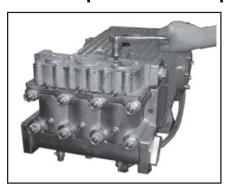
1) Remove socket head cap screws (58)
