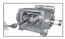
12) Remove the connecting rod screws (24). Important! Connecting rods are marked 1 to 3 for identification. Do not rotate connecting rod halves or interchange them. When reassembling, the connecting rod must be fitted in their exact original position on the crankshaft journals.
