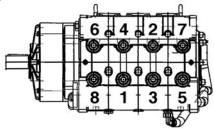
Important! The torque tension on the screws (49A) must be checked after 8-10 operating hours; the pump must be at zero pressure. Thereafter, the tension is to be checked every 200 operating hours.
