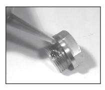
Remove the o-ring (31). Inspect all parts for wear and replace as necessary. Apply one drop of loctite 243 to the valve plugs (32) and tighten to 125 ft. lbs.
