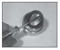
8) Remove the weep grooved seal (23B) together with pressure ring (24) out of the seal case (20). Check O-rings (21).
