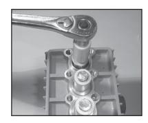
10) If the plunger pipe (16B), or oil seal (19) is worn, removetension screw (16D) and remove along with plunger pipe (16B). Check and clean plunger surface (16A), check oil scraper (16H). Remove the gear seal adapter (20A) and, if necessary, replace oil seals with seal lops facing crankcase (1). If the gear seal adapter is removed, replace the o-ring (22). Cover thread of tension screw (16D) with a thin film of Loctite and tighten carefully to 26 ft.-lbs. (35NM).
