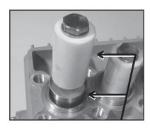
Check surfaces of plunger (16). damaged surfaces cause accelerated seal wear. Deposits of all kinds must be removed from the plungers.
