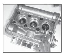
7) Remove the pressure rings (24) and grooved seals (23) from the valve casing (26).
