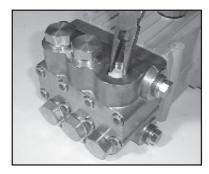
Using needle nose pliers, remove the inlet and discharge valve assemblies (27-33). Note: It may become necessary to remove the valve seat (27) from the valve casing using a slide hammer.
