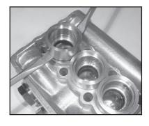
Remove seal case (20) and weep return rings (25) from the valve casing.
