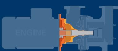
This double oil bath seal is able to avoid dry running of the seals when the pump is priming. Thanks to this seal, less maintenance is carried out and more reliability is given.
