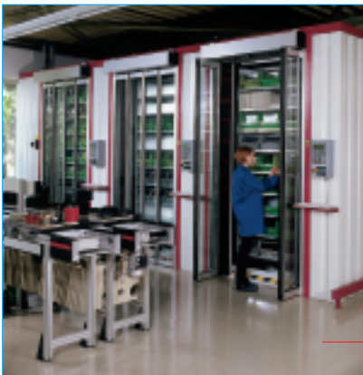
The modules are called forward from the central storage system on an order-specific basis
