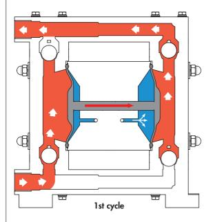
REKO-FLUX air-operated diaphragm pumps are positive displacement pumps consisting of two pump housings and one control valve part. Diaphragms within the pump housings securely separate the liquid section (red) from the air section (blue). Both diaphragms are connected by a selector shaft which is located in the control valve part.
