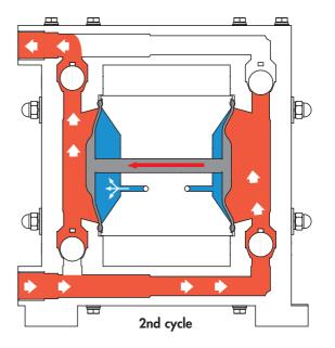
Compressed air inflating alternately the air sections causes a movement of the diaphragms (1st and 2nd cycle). The subsequent transfer operation is controlled by a control valve which is easy to dismantle.
