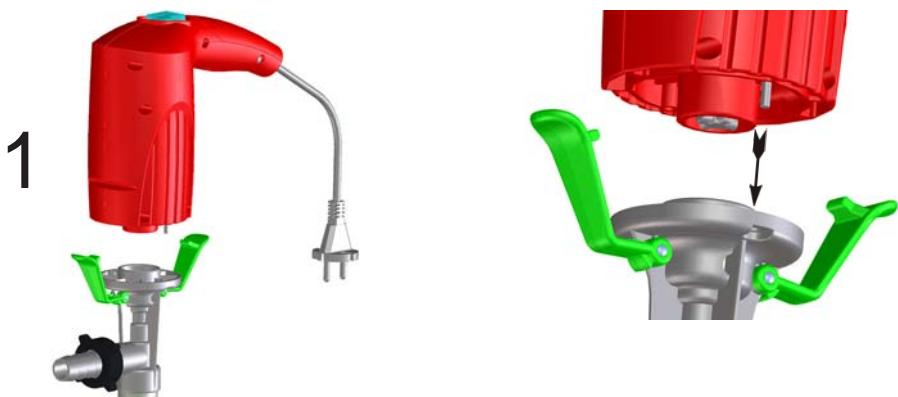
Position the motor in such a way that the pin fits into
