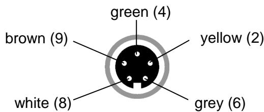
The shielding is lead through on „black“ at the cable.
