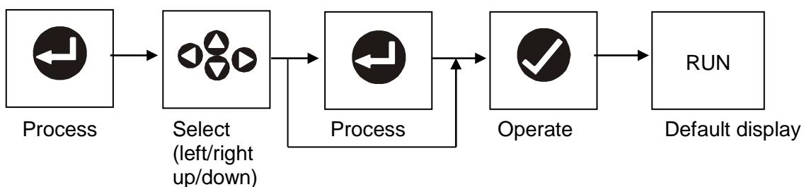
The current and possible settings can be quickly seen by feedback in the Info line and by the flashing symbols.
