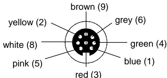
The shielding is lead through on „black“ at the cable.
