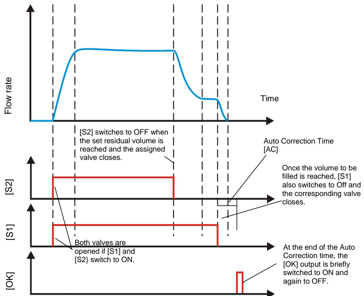
Should the measuring unit fail during the filling process and should no more pulses be generated, the valve would no longer be able to close.
