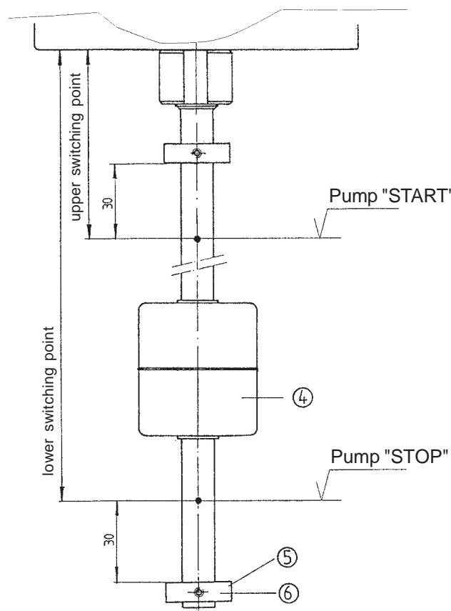
Cautiously push both cords brown-blue ( lower switching point "STOP" pump ) onto the already set lower switching point until the relay will be released.
