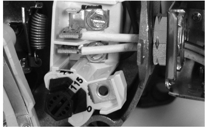
Figure 17 - Voltage set to 115 V, Dial Type
