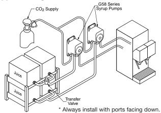
The diagram above shows a "typical Bag-in-Box installation" with a single bag connection and a multiple bag connection with a Flojet Transfer Valve assembly. Flojet Part Nos. 1500-031 and 1500-131 transfer valves are recommended for automatic unattended change-over from empty to full bag for all G58 pumps.
