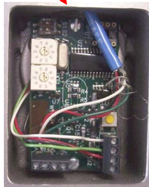
Optional SCL signal conditioner Not yet approved for use in the EU.
