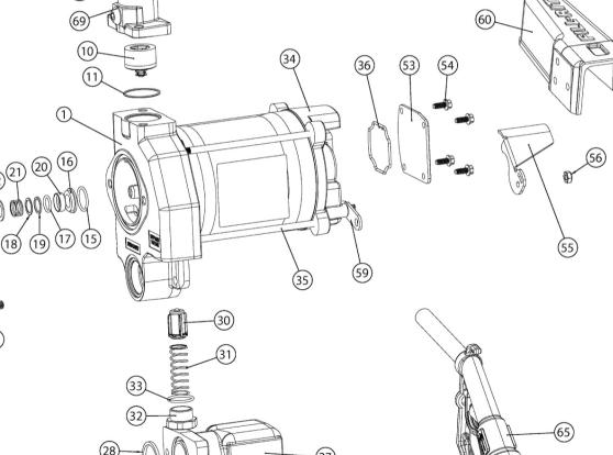
\*KIT700BD is for conversion of pump for use with Biodiesel products. In this kit, the wetted materials listed above are changed to VITON and Fluorocarbon seals to allow for compatibility with Biodiesel products.
