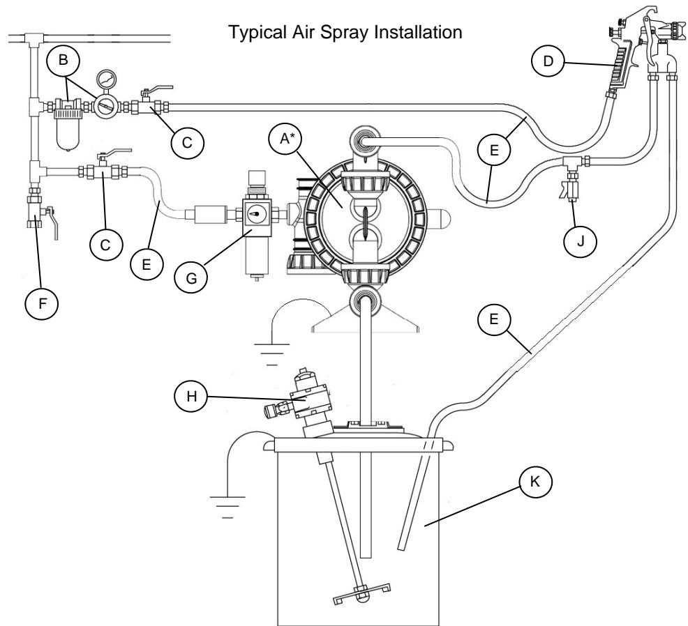
\*NOTE: Mount pump securely to a solid surface using appropriate bracketry and attaching hardware for the application.
