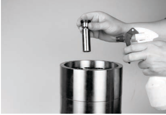
21. Spray with water and mount pistons
