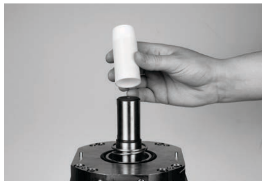
40. Mount special tool on shaft
