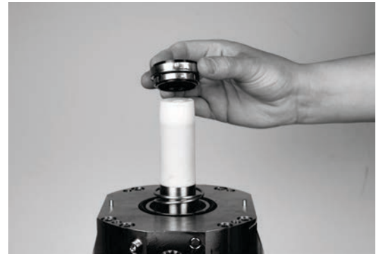
42. Mount sealing (smallest diameter pointing down)
