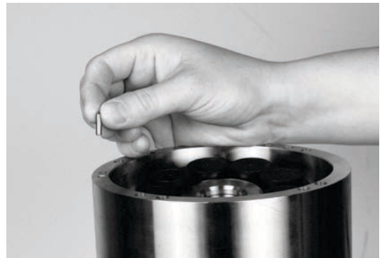
27. Mount 1 guide pin on housing
