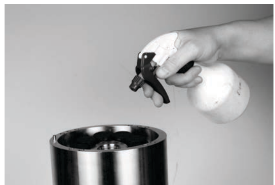
28. Spray piston shoes with water
