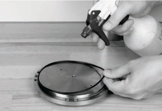
22. Spray with water and mount O-ring on end cover
