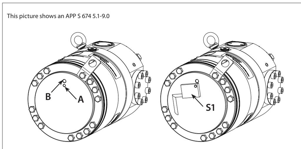
All APP S 674 pumps are designed with M6 and M8 threads for mounting the temperature sensor. The threads are placed differently depending on pump size.
