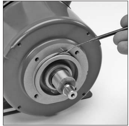
6.3 Lubricate and install o-ring (12) onto motor flange.
