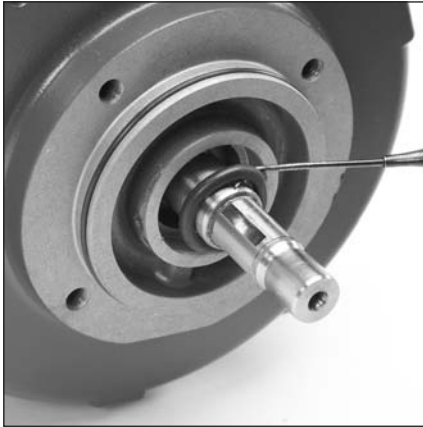
5.8 Remove and inspect slinger o-ring (11) from motor flange.
