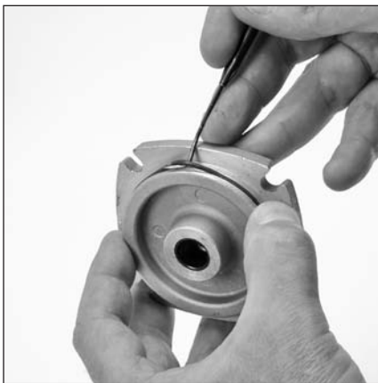
6.7 Lubricate and install o-ring (6) onto bearing cover (5).
