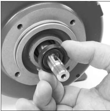
5.7 Remove and inspect shaft seal (10) from motor flange. Do not scratch or damage motor shaft surface. (See Note)
