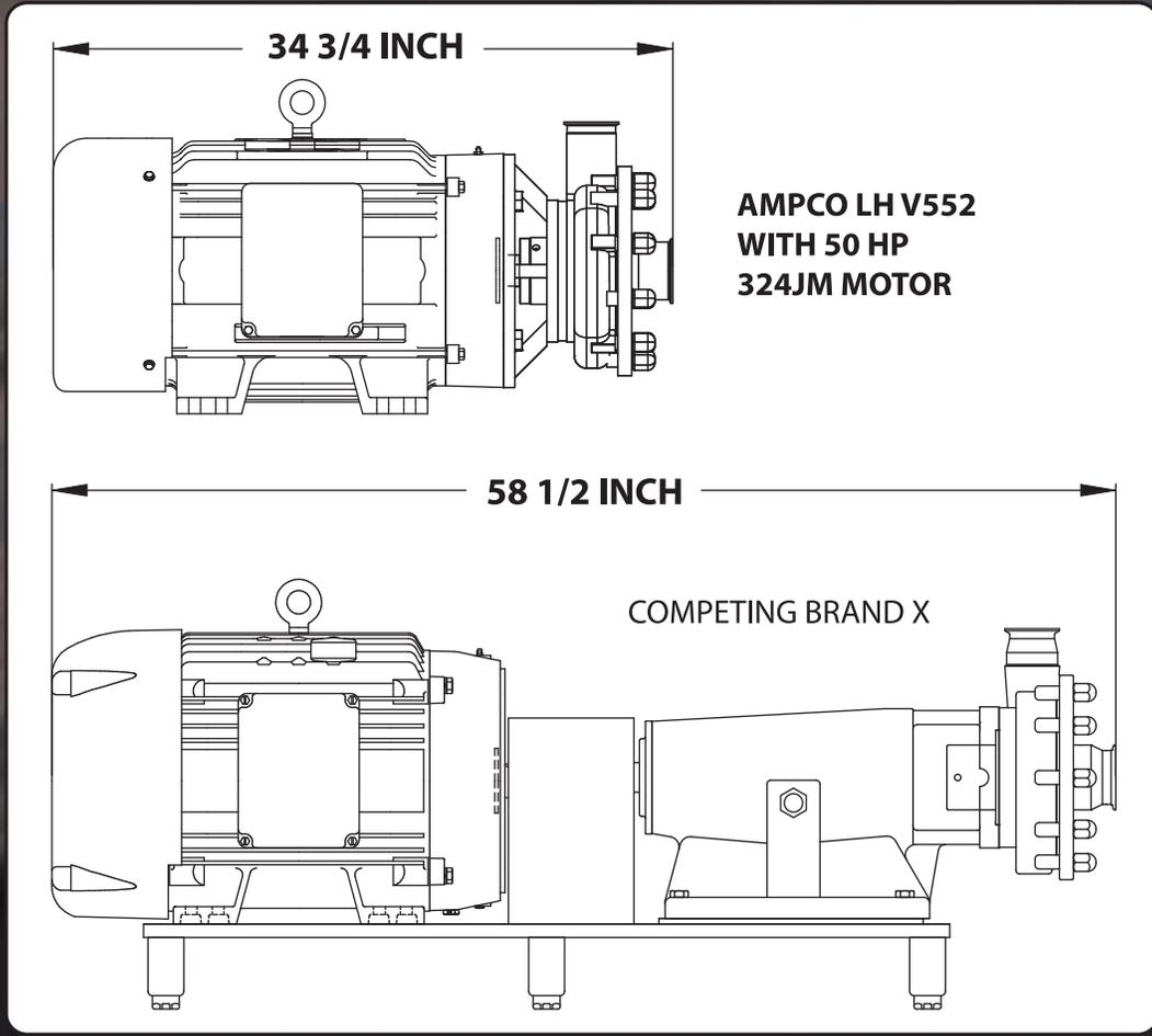
**LH Pumps are available in 3 models ranging from 15 HP to 75 HP**
