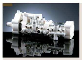
The Fluid Powered Proportioning Pump FPP series, developed by Fluid-o-Tech, is designed to mix two different fluids with a high degree of accuracy. The pump operates thanks to the energy stored in any pressurized fluid, which gives power to the unit. The mixing ratio, determined by the dimensions of the two chambers, is constant regardless of the flow rate and pressure requested by the application. The food grade materials used in the pump, have a high degree of compatibility.
