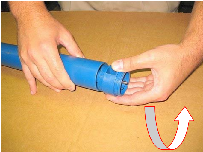
Reinstall the impeller housing cover by turning counterclockwise
