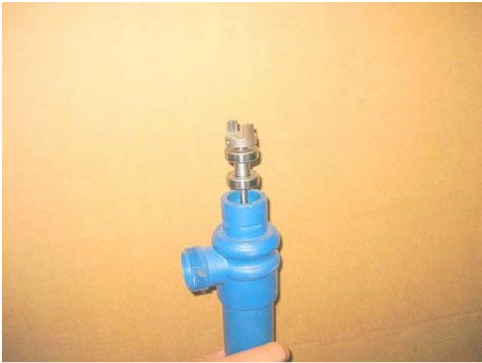
Picture illustrating bearing completely removed from pump head.
