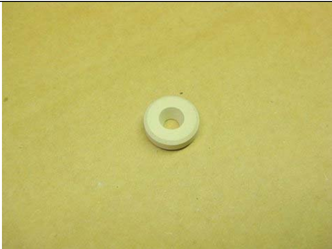
Top view of new seal (tapered side)
