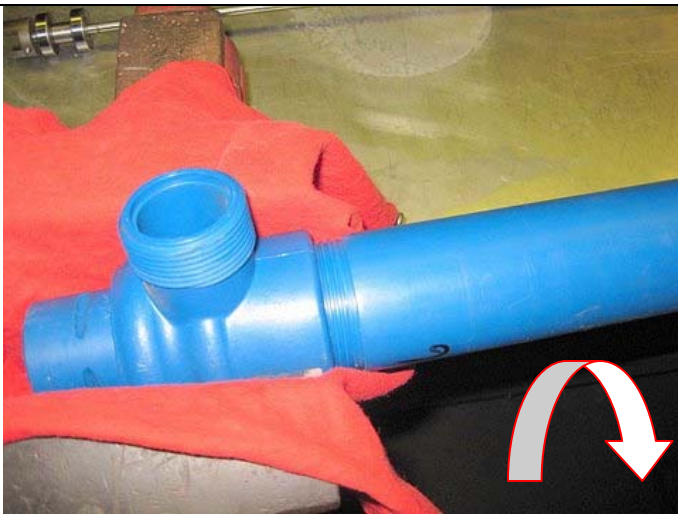
Place pump head in a vise and remove the intake tube by unthreading clockwise.
